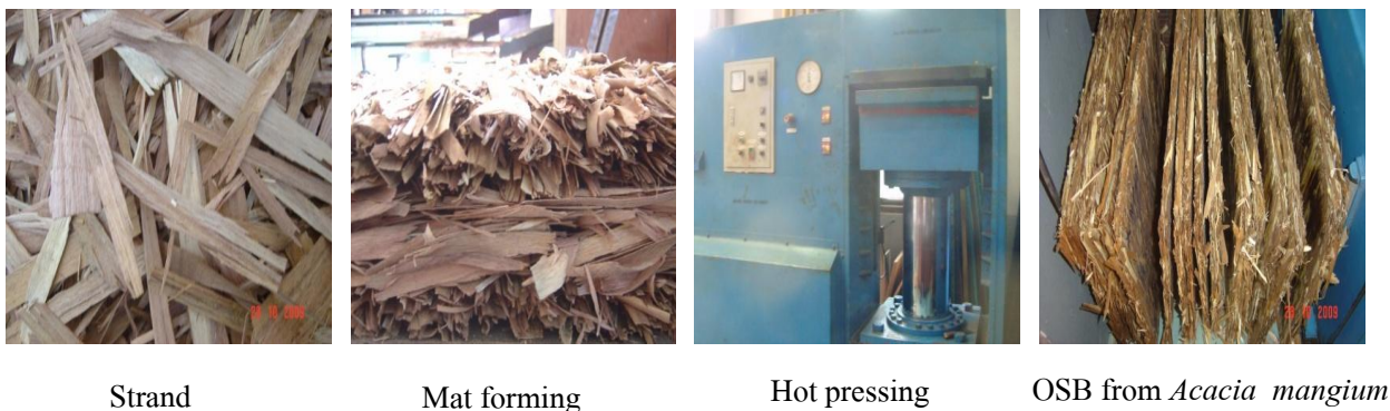
Figure 3. Production of Oriented Strand Board (OSB) from Acacia mangium .
