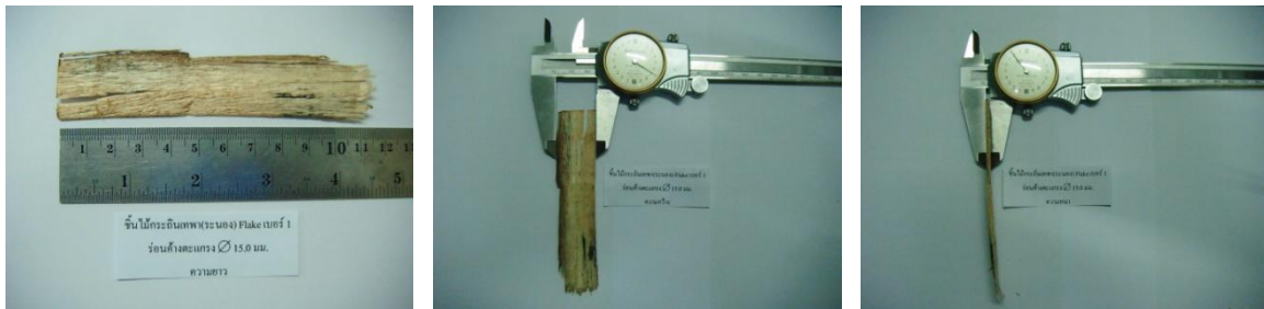
Figure 5. Measuring strands of Acacia mangium .
